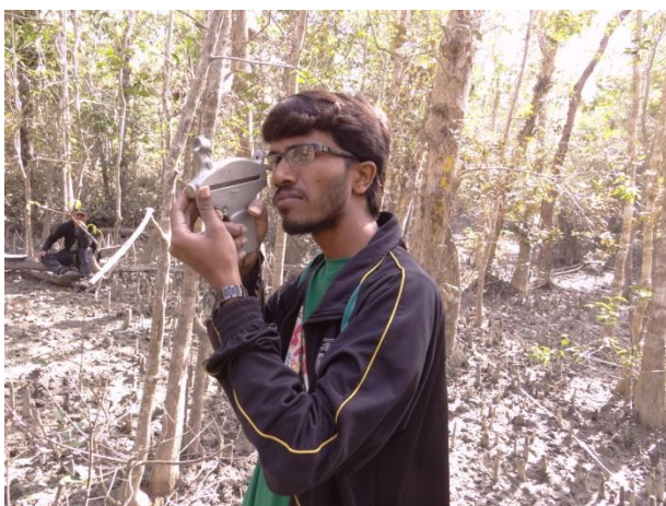
Measuring tree height with The Haga altimeter
