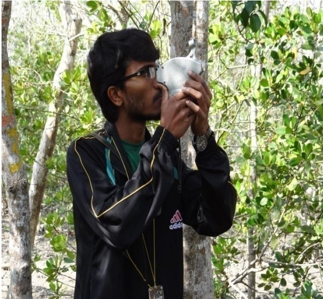
Photo 11.1: Surveyor measuring tree height using Hoga Altimeter in January 2015 monitoring
