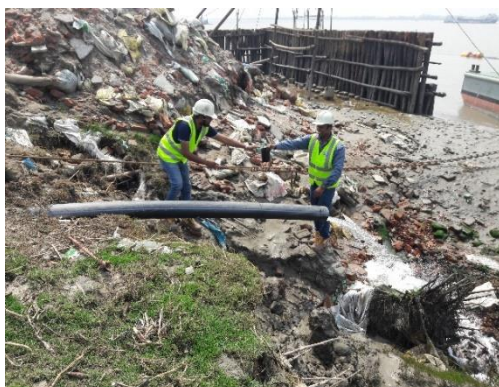
Figure 2.4: RO Discharge Water Sample Collection and Discharge outlet
