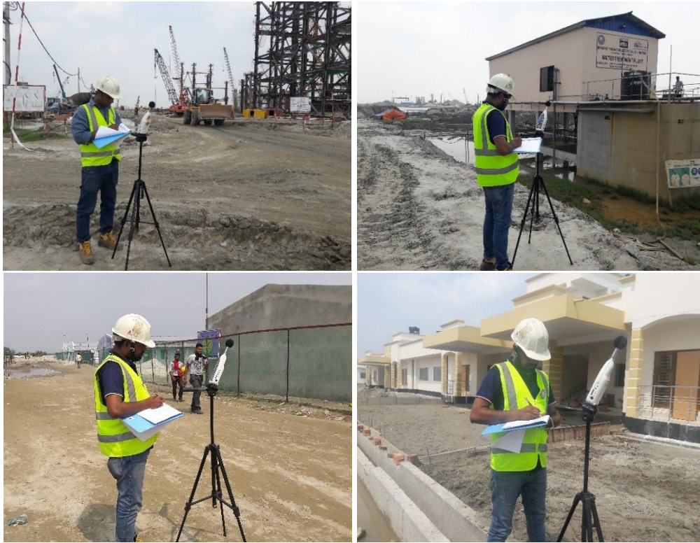
Figure 2.7: Ambient Noise Level Monitoring during Day Time
