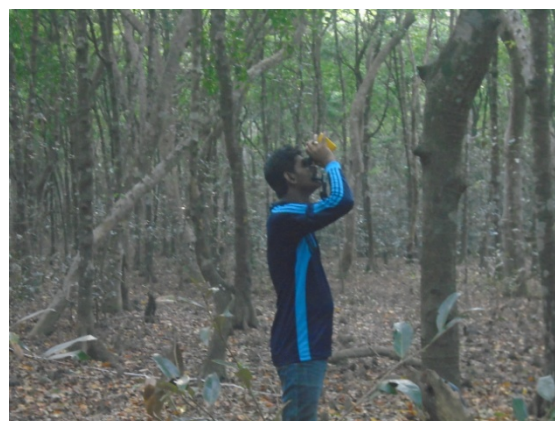
Photo 3.3.10: Team member measuring the height of tree using Range finder
