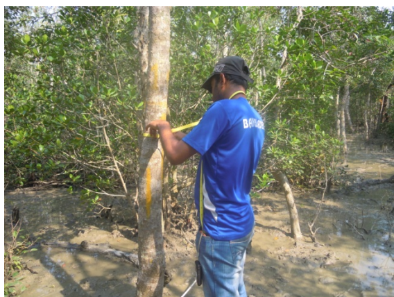
Photo 3.3.9: Team member measuring the DBH of tree using Diameter tape
