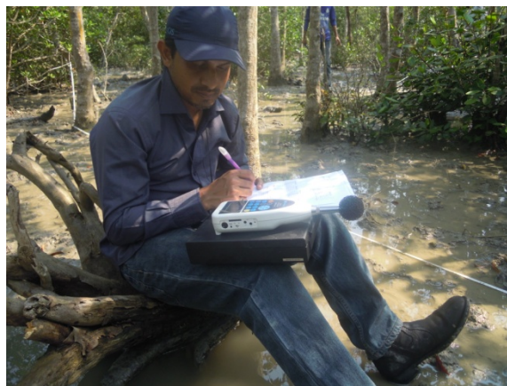
Photo 2.2.1: Professional conducting an ambient noise acquisition survey
