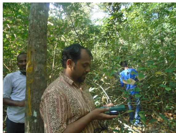
Photo 3.3.8: Team member taking light intensity using Lux Meter
